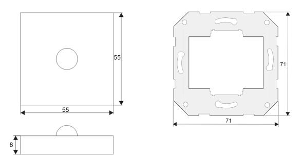
Notice: Outside dimensions are depending on the frame used of the respective switch ranges.
