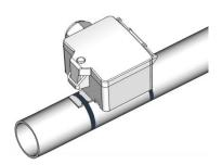
For detection of water condensation, the sensor must be mounted on the coldest point of the medium. Please ensure a good thermal contact to the measuring medium. A thermal connection between sensor und medium with heat conducting paste is necessary. Mounting effects by means of included cable ties (binders). Mounting can be made directly on a pipeline.
