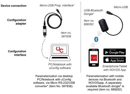
\*Commercially available Bluetooth dongles or USB to Micro-USB adapter cables are not compatible. You need a mobile device that supports at least Bluetooth version 4.1. The configuration app with the corresponding instructions can be downloaded from the Google Play Store or the Apple App Store.
