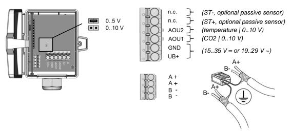
The modbus address of the device is set in the range of 1 ... 31 (binary encoded) using a 5-pole DIP switch. With address 0 via DIP, an extended address range (32..247) is available via USEapp.
