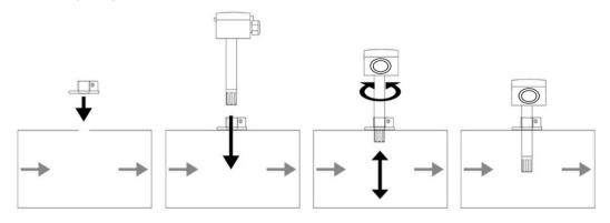
Maximum air speed 10 m/sec. Fix mounting flange at the air duct, fix the sensor at the mounting flange.
