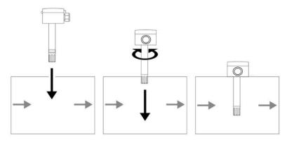
Maximum air velocity 10 m/s. Fix the sensor at the air duct.
