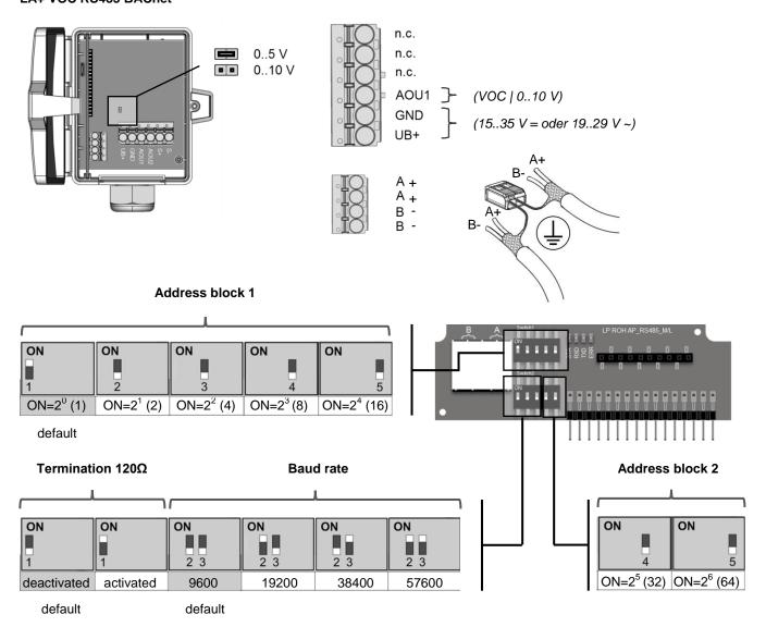
The BACnet address of the device is set binary coded in the range of 1 ... 127 via 7 dip-switches. (the address 0 is reserved and cannot be selected).
