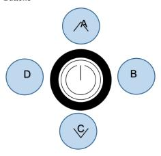
The configuration menu is called up by simultaneously pressing the buttons "up" (A), "left" (D) and "right" (B) for at least 3 seconds.
