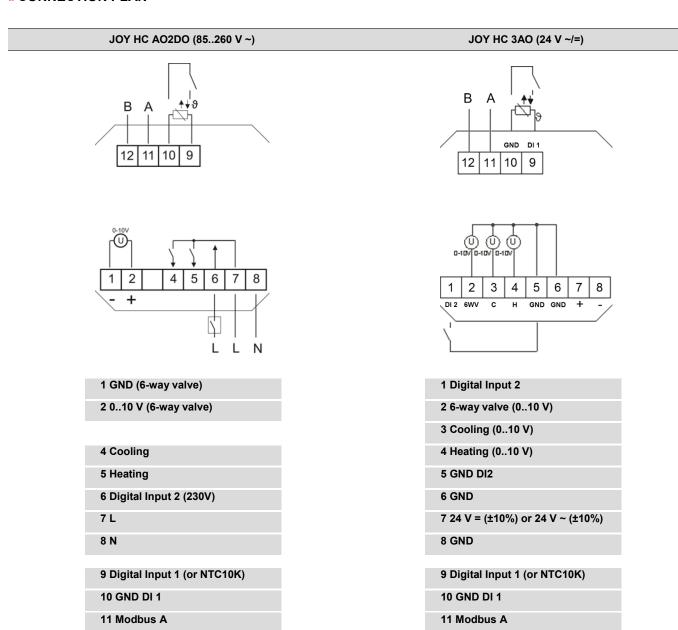
Note: Parallel connection of the potential-loaded inputs is not permitted!
