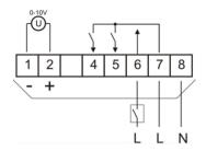
1 GND (6-way valve) 2 0..10 V (6-way valve)
