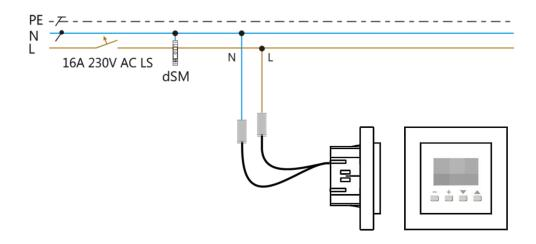
After the electrical connection has been established and the power switched on, the device is automatically registered at the digitalSTROM meter in the electric circuit distributor. The device is then immediately ready for operation, begins with the recording of the room temperature and humidity and registers these in the digitalSTROM system.
