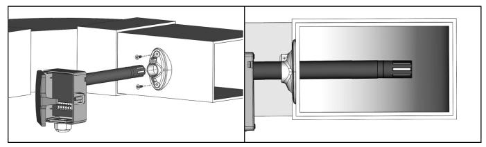
Optional mounting with mounting base (Item No. 631228), please note the installation depth of the sensor pipe.
