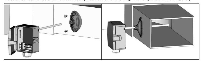
Optional mounting with mounting base (Item No. 631228), please note the installation depth of the sensorpocket. (permissible ambient temperature -35..+70 °C)
