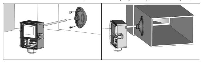
Optional mounting with mounting base (Item No. 631228), please note the installation depth of the sensorpocket. (permissible ambient temperature -35..+70 °C)
