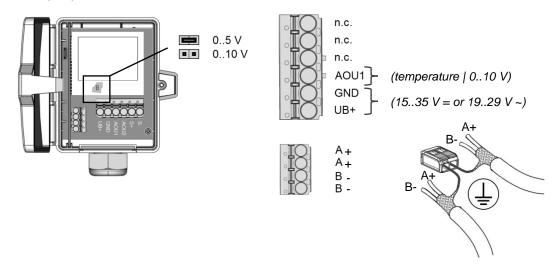
The BACnet address of the device is set binary coded in the range of 1 ... 127 via 7 dip-switches. (the address 0 is reserved and cannot be selected).
