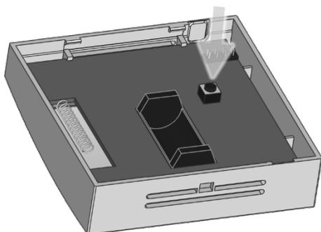
After delivery the room operating unit might be in default shipping mode, in this case press the learn button (<1 second) at the rear of the device [Signal telegramm will be send, SIG -> 0x0F // shipping mode deactivated].
