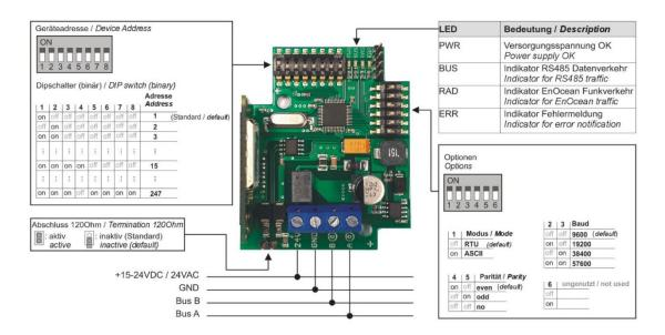
When using ASCII mode, the parity must be set to EVEN or ODD. "No Parity" (no) is not available in ASCII mode.
