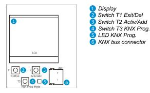
This device is powered only by the KNX bus.
