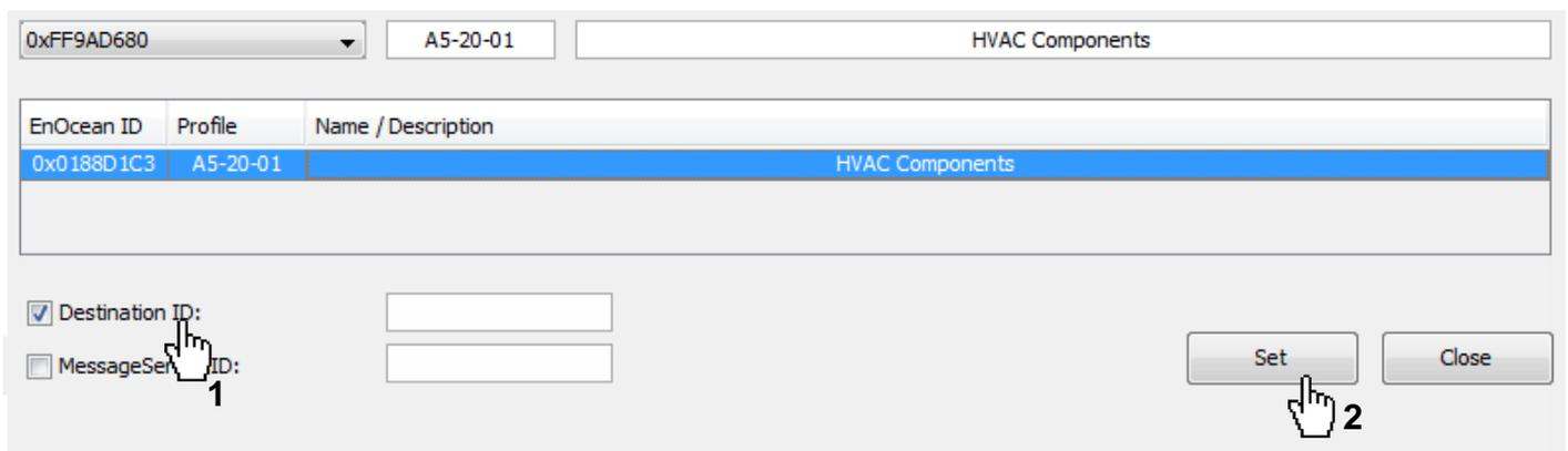
Send the new configuration to the BACnet IP Gateway. A click with the right mouse button on the device symbol opens the context menu. Select the **<Send configuration>** entry. A restart of the device is not required. When the configuration process is completed, the configuration session has to be closed with the **<End LEARN mode>** entry.
