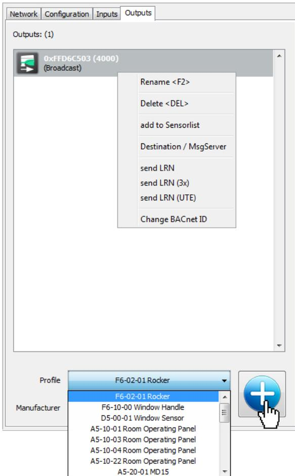
Click right on a particular sensor icon to open the context menu and select **<send LRN>** to send a Learn-in message to the device that is to be paired with this message.
