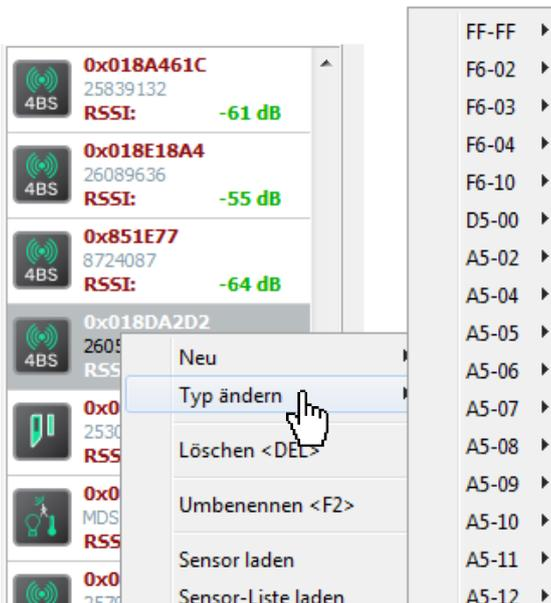
If the EEP of a particular sensor is already known, the EEP can be set manually by clicking right on the sensor's icon and selecting the EEP from the "change type" dialogue.
