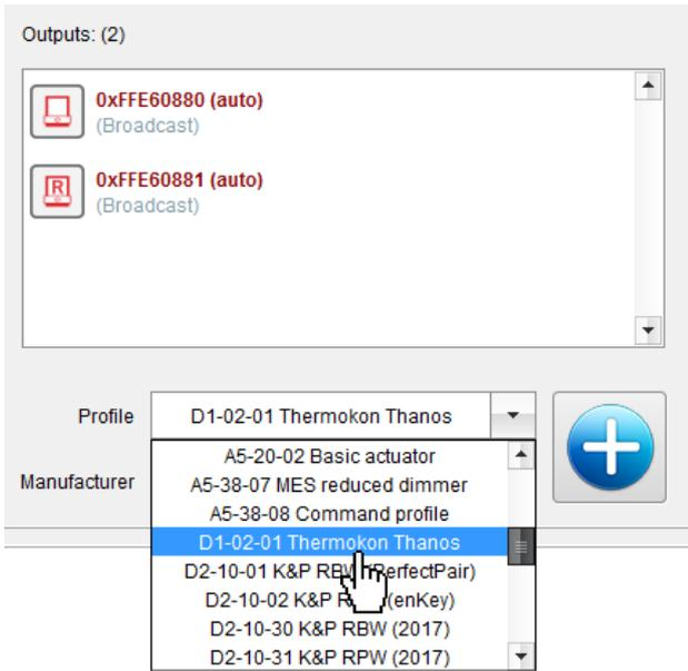
thanos does require a bidirectional teach-in as well to receive data from thanos but to change settings in thanos as well. Select thanos in the output section and add it to the outputs. You will see that 2 icons will be created, one for requesting data and one for sending commands to thanos.
