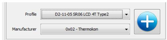
Select the appropriate profile on the „Outputs“ tab. Add the profile to the “outputs” using the blue plus symbol.
