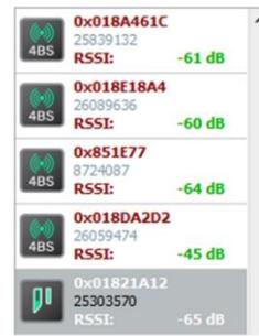
The Inputs section shows the EnOcean devices that will be converted into BACnet data points. To generate data points the gateway needs to know the sensor's EEP as this defines what data point will be created. Therefore only EnOcean sensors which have been recognized can be assigned. Sensors with icons indicate the type of message only (i.e. 4BS, VLD, MSC) cannot be assigned and will be highlighted in red to indicate the problem.
