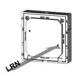
After delivery the room operating unit might be in default shipping mode, in this case press the learn button (<1 second) at the rear of the device [Signal telegramm will be send. SIG -> 0x0F // shipping mode deacticvated].
