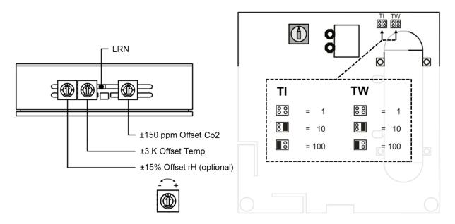
Pre-setting: (TW) T\_wake up: 100, (TI) T\_interval: 10
