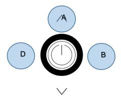
The configuration menu is called up by simultaneously pressing the buttons "up" (A), "left" (D) and "right" (B) for at least 3 seconds.
