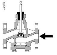
**Special version VVF52..G** for saturated steam, super-heated steam up to max. 600 kPa (6 bar) abs
