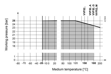
Working pressure and medium temperature staged as per ISO 7005
