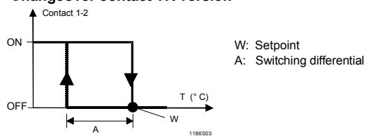
If the probe has cooled down to a temperature below approx. -20°C, the control current circuit opens, however, automatically closes again, when the temperature rises.
