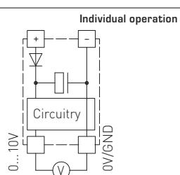
When several devices are supplied by one 24 V AC voltage supply, it is to be ensured that all "positive" operating voltage input terminals (+) of the field devices are connected with each other and all "negative" operating voltage input terminals (-) (= reference potential) are connected together (in-phase connection of field devices). All outputs of field devices must be referenced to the same potential!
