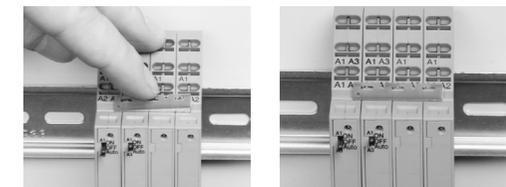
The tails of the connecting bridge carry potential, therefore place the bridge in the middle of the aligned modules to eliminate any accidental touch.
