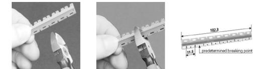
Cut the needed number of contacts with wire cutting pliers at the respective predetermined cutting point. Then insert the connecting bridge from the top into the contact slot and press it downwards into place.
