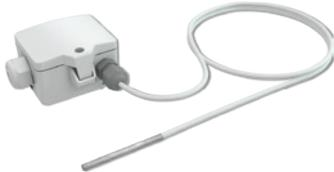
Cable sensor for temperature measurement in HVAC applications. Depending on the application requirements, different PVC, silicone and PTFE cables are available. A hinged cover and tool-free wiring as well as removable cable entries ensure a quick and easy installation. The TF14 with its 4 mm diameter pocket is well suited for fast response applications.
