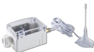
The SRE-Repeater is used for repeating radio telegrams between EnOcean transmitters and receivers/gateways. The repeater is typically used when transmission range problems occur between transmitter and receiver in an existing installation (e.g. due to walls being pulled in, furniture/cabinets being moved). Level 1, Level 2 and Smart Repeating (rule-based filters) can be set using the free airConfig software. Ideal for installation in suspended ceilings.
